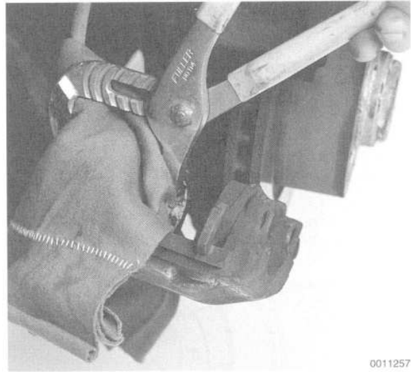
Fig. 6. Brake caliper piston being pressed into caliper. Use a rag to protect caliper piston and seals.
