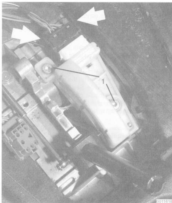
Fig. 8. Disconnect harness connector by pressing connector retaining clips together (arrows). Switch mounting screws shown at 1.
