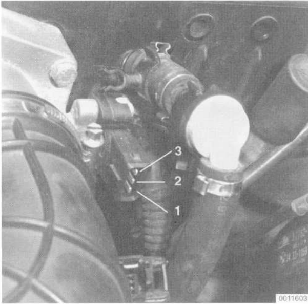
Fig. 9. Throttle position sensor terminal identification on M50 engine.
