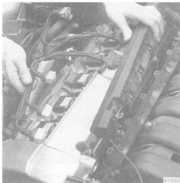
Fig. 11. Main harness being lifted off engine to be placed at base of windshield.
