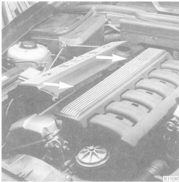
Fig. 8. Remove top engine cover by prying out plugs and removing nuts (A). Make sure rubber insulators (quantity 4) on either side of cover do not fall off during cover removal (arrows).
