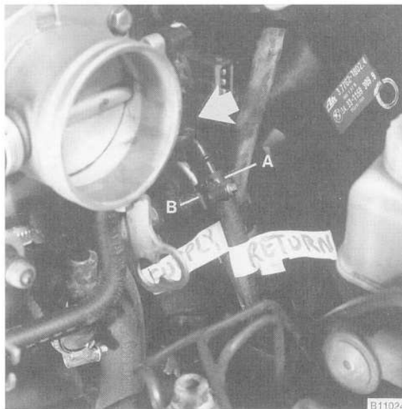
Fig. 18. Fuel return line (A) and fuel supply line (B). Label fuel lines before disconnecting them. Remove bracket mounting to free lines (arrow).
