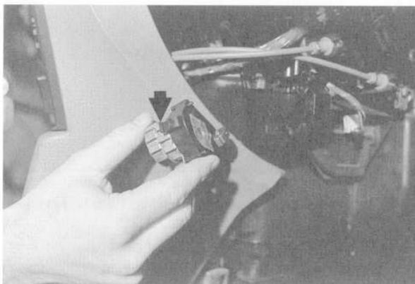
Fig. 16. Air distribution flap stepper motor mounting clip (arrow). Release clip and tilt motor out of housing.
