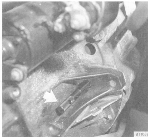
Fig. 20. BMW special tool 11 2 300 inserted through bellhousing hole and into flywheel (arrow).
