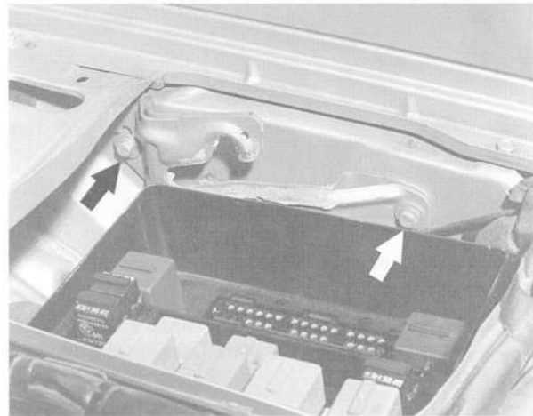
Fig. 8. Hood rear catch mounting bolts (arrows). Loosen bolts to reposition catch.
