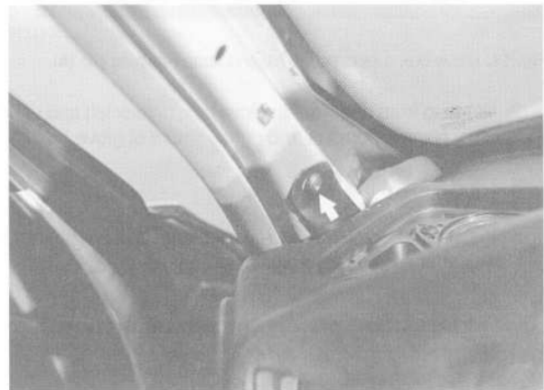
Fig. 9. Instrument panel mounting screw (arrow) in left side A-pillar.
