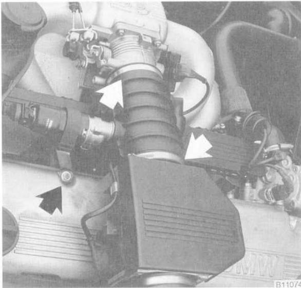
Fig. 26. Idle speed control valve (arrow).
