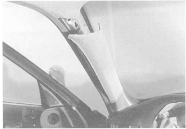
Fig. 8. A-pillar interior trim panel shown removed.
