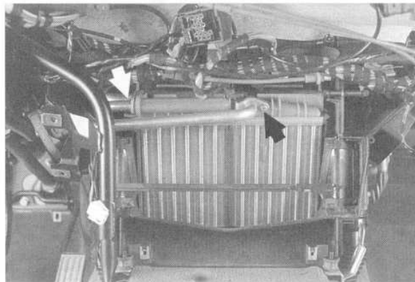
Fig. 11. Heater pipe mounting bolts on heater core (arrows).
