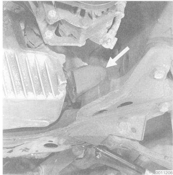
Fig. 17. Left lower engine mount (arrow).
