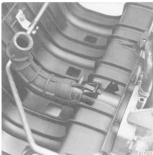
Fig. 17. Idle air control hose at underside of intake manifold. Carefully depress clip (arrow) and pull out hose fitting.
