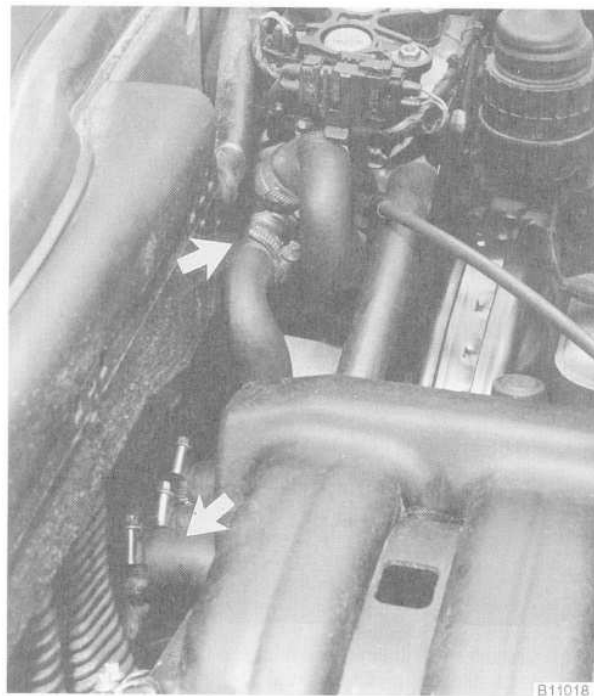
Fig. 12. Heater hoses at bulk head and heater valve (arrows) to be disconnected.
