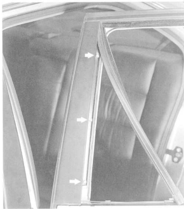
Fig. 7. Outside trim cover mounting screws (arrows). To remove cover slide up and then off door.
