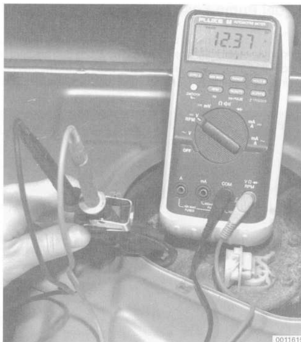
Fig. 9. Voltage supply to fuel pump being checked at harness connector terminals 4 (–) and 5 (+).
