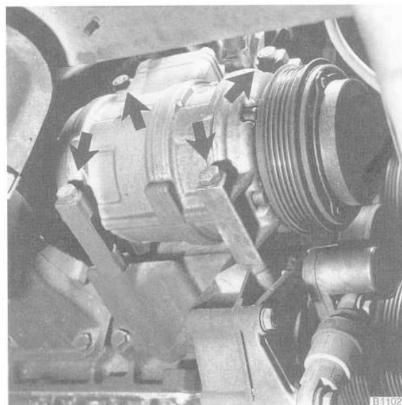
Fig. 20. A/C compressor mounting bolts (arrows).
