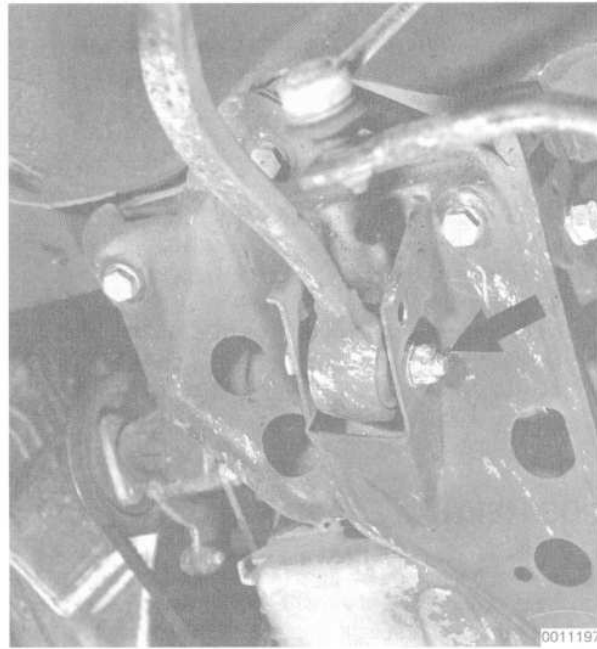
Fig. 9. Control arm through-bolt (arrow).
