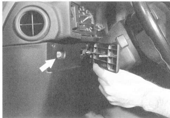
Fig. 12. Lower instrument panel trim cover being removed on cars with SRS airbag. Pry cover out of clip (arrow), then slide cover outwards toward left.
