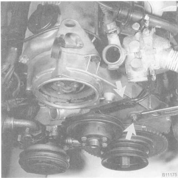
Fig. 9. Upper alternator bracket nut and wiring duct (arrows).
