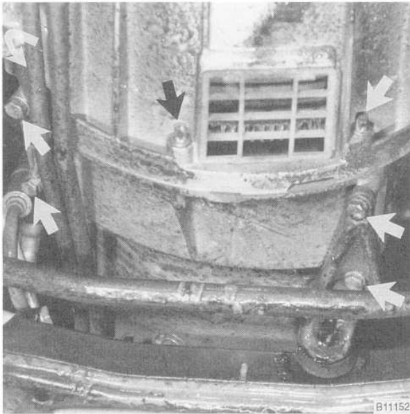
Fig. 4. Bellhousing reinforcement plate mounting bolts (arrows).
