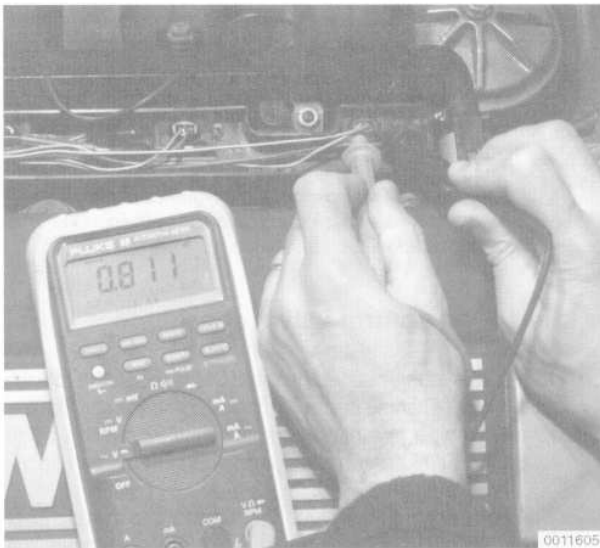
Fig. 13. Voltmeter connected across fuel injector connector with engine running (M50 engine shown).
