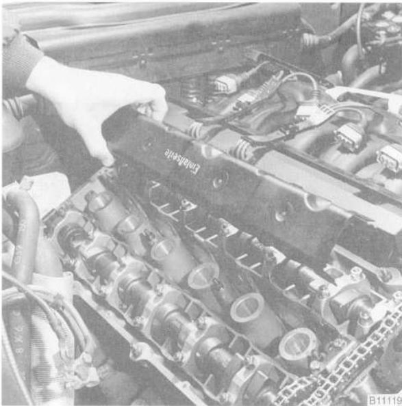
Fig. 5. Oil baffle cover being removed.
