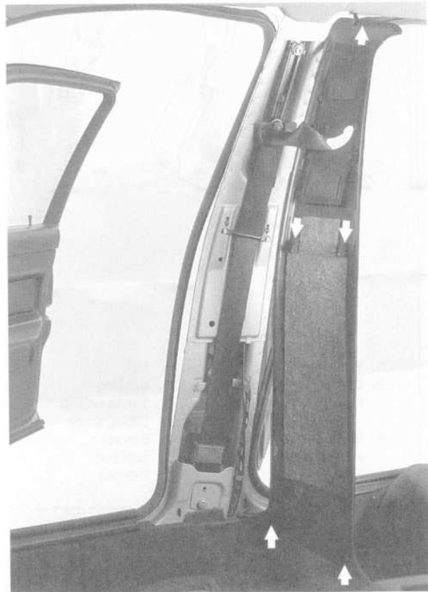
Fig. 1. B-pillar trim panel retaining clips (arrows).
