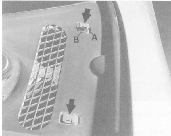
Fig. 9. Moulding grille retaining clips (arrows). Remove clip center piece (A) from outer piece (B).
