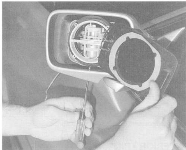
Fig. 5. Screwdriver inserted into opening in mirror housing. Pivot screwdriver away from door to unlock glass. Pivot screwdriver towards door to lock glass.
