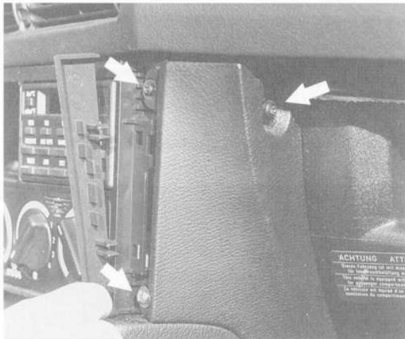
Fig. 4. Plastic trim panel being removed (1991 and later cars only). Trim panel mounting screws shown at arrows.
