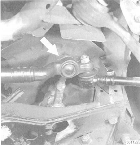
Fig. 8. Idler arm-to-center tie rod self-locking nut (arrow).
