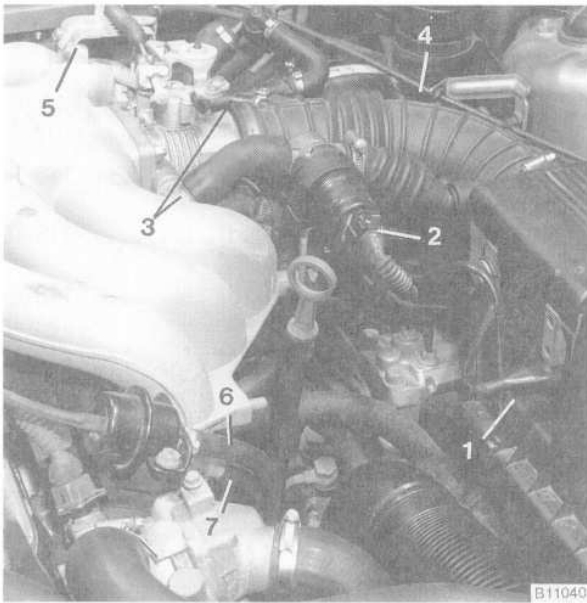
1. Air flow sensor connector 2. Idle control valve connector 3. Vacuum hoses 4. Intake air duct 5. Throttle, accelerator, and cruise control bracket 6. Fuel return hose 7. Fuel supply hose
