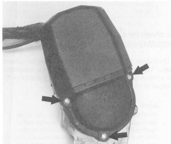
Fig. 5. Distributor cap mounting screws (arrows).
