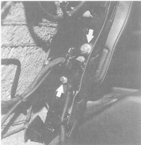
Fig. 4. Front seat armrest mounting nuts (arrows).
