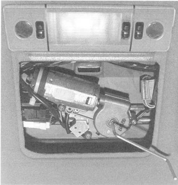
Fig. 3. Use hex key to manually close sunroof. Turn hex key counter-clockwise to manually close sunroof.
