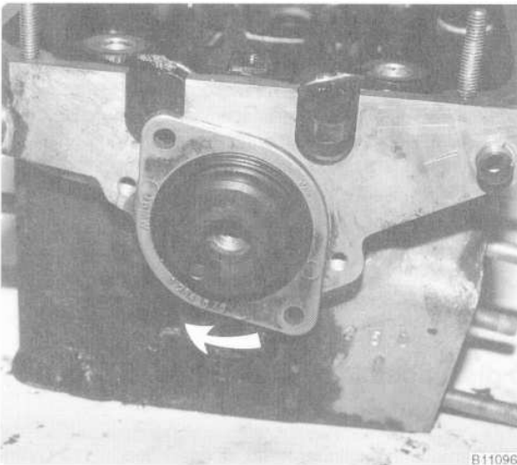
Fig. 18. Camshaft oil seal housing at front of cylinder head. Rotate oil seal carrier during removal (arrow).
