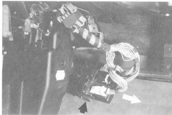
Fig. 31. Depress clip (bottom arrow) and slide control module out.
