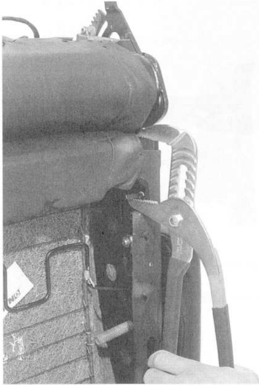
Fig. 11. Release seat back locking lever using pliers.
