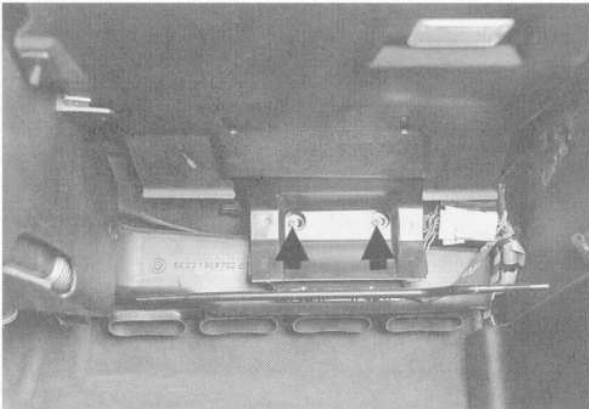
Fig. 6. Ventilation air duct retaining screws (arrows).
