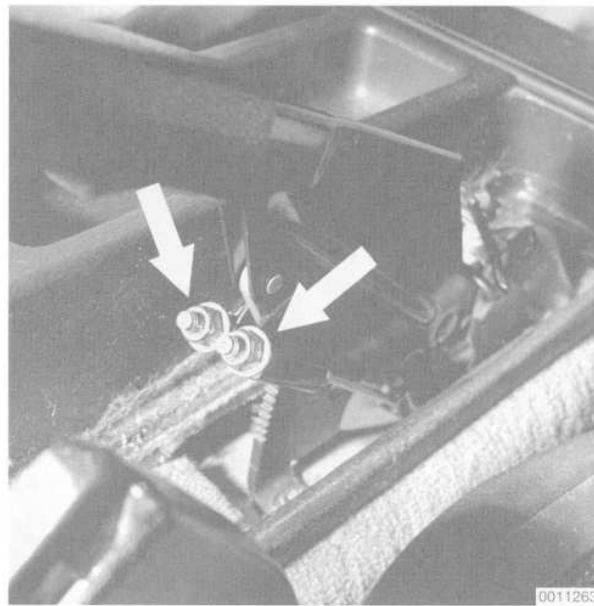
Fig. 16. Parking brake cable adjusting nuts (arrows).
