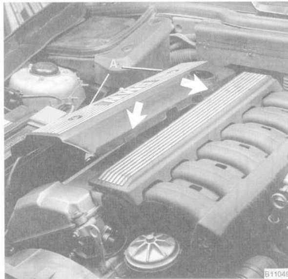
Fig. 27. Remove top engine covers by prying out caps and removing nuts (A). Note rubber gaskets at cover edge (arrows).
