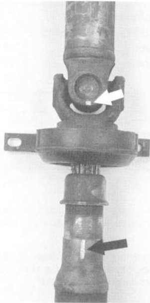
Fig. 11. Before pulling apart driveshaft sections, make matching marks as shown.
