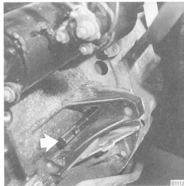
Fig. 11. BMW special tool no. 11 2 300 installed through bellhousing and into flywheel.
