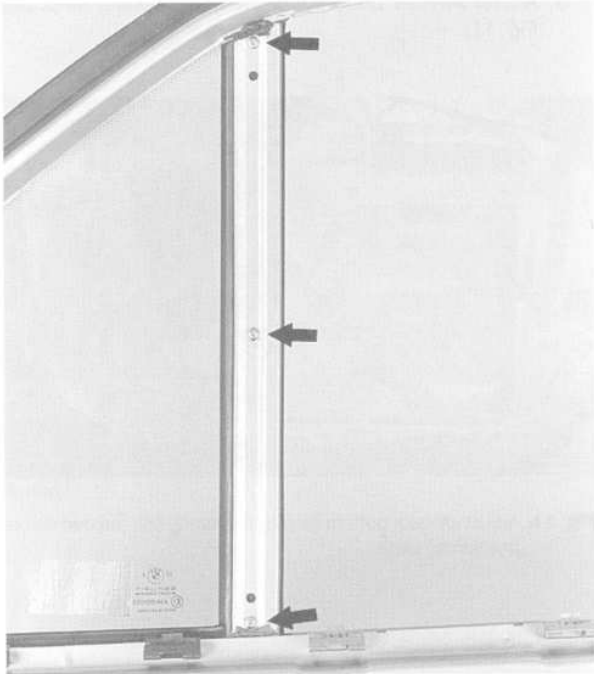
Fig. 6. Rear window guide mounting screws (arrows).
