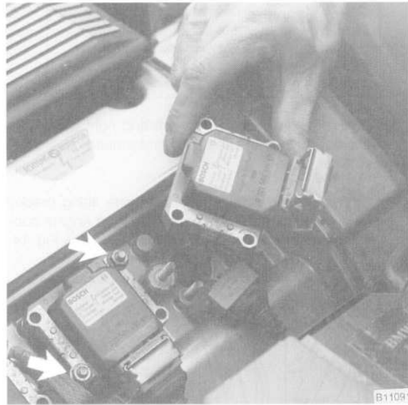
Fig. 12. Ignition coil being removed.
