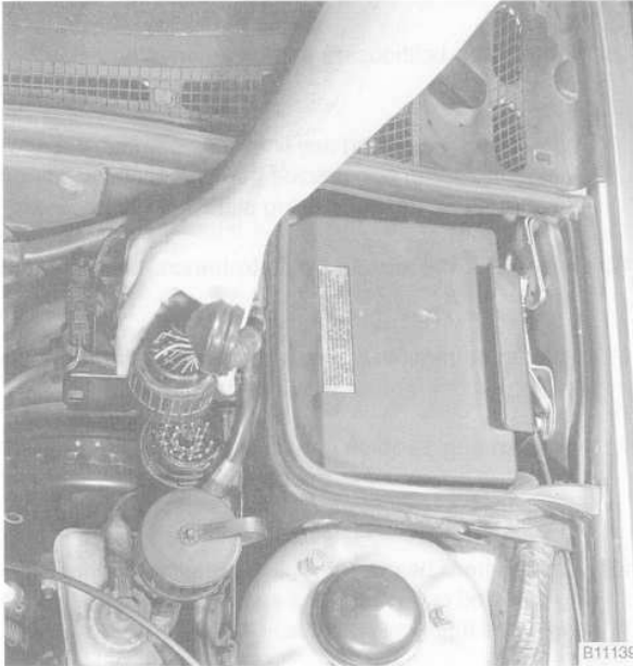
Fig. 2. Main harness connector being separated at bulkhead on 525i model.
