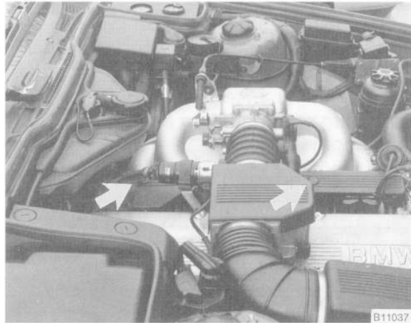
Fig. 29. Wiring harness bracket cover plugs (arrows).
