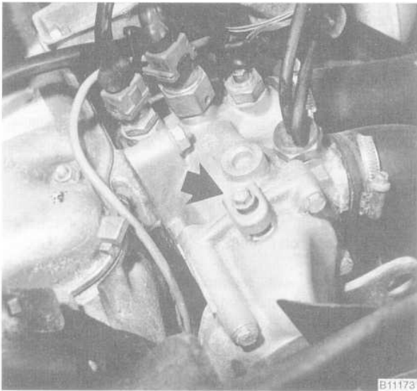
Fig. 7. Cooling system bleed screw (arrow) on 535i model.
